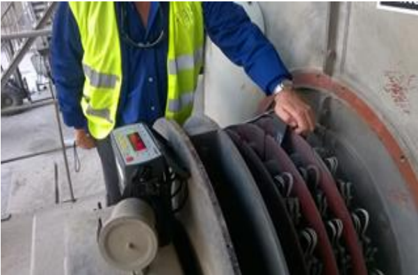
Fig. 12 Measurement of the resistive unbalance in the rotor winding with a digital microhmeter.
