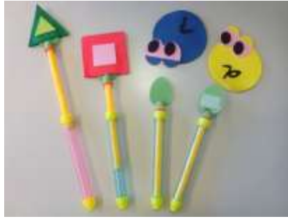
Figure 3. Extendable robot control paddles. From left to right: shift forward, stop, turn left, turn right
