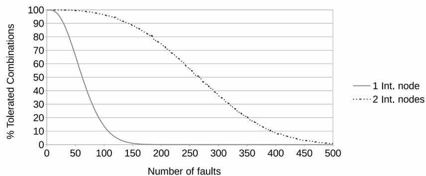
Figure 6. Fault combinations tolerated by the methodology when using one or two intermediate nodes in a 3-D network with 1,000 nodes.
