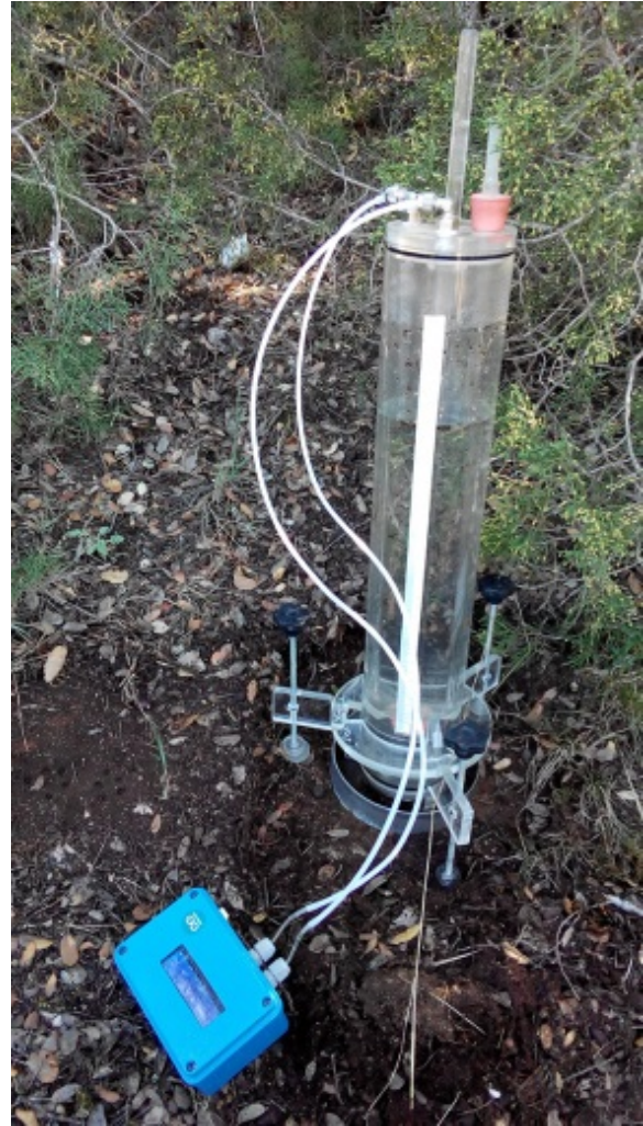
Fig. 3. Compact automated infiltrometer proposed by Di Prima (2015). The device consists of a containment ring with a small head of water that is controlled by a Mariotte reservoir and a data acquisition system based on the open source microcontroller platform Arduino.
