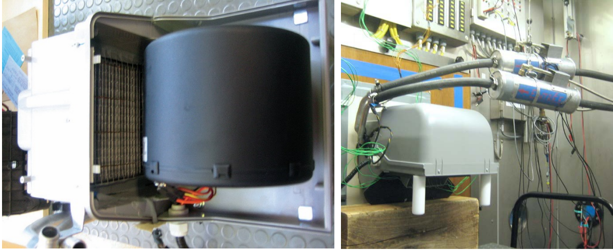
Fig. 4. Experimental setup: HEX inside the HVAC unit (left) and HVAC unit on the test bench (right).
