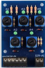
Fig. 7. Simulator for 5 analogue inputs
