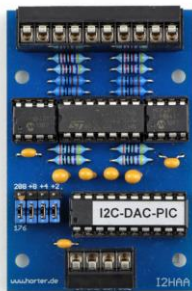
Fig. 6. Analogue output card 12 bit
