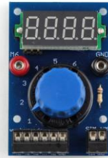
Fig. 8. Simulator for 6 different analogue values
