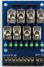
Fig. 9. Simulator for 8 digital inputs
