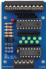
Fig. 3. Digital input card 8 bit
