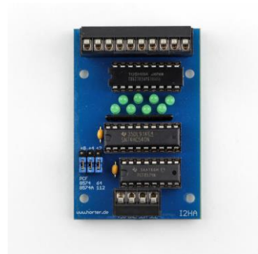
Fig. 4. Digital output card 8 bit
