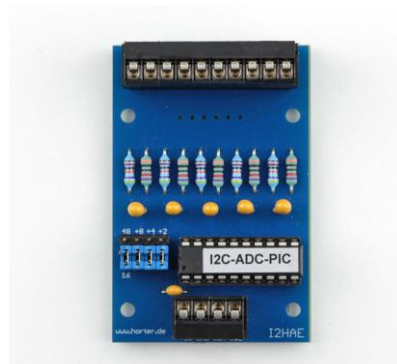
Fig. 5. Analogue input card 12 bit
