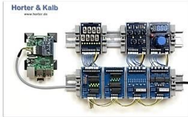
complete PLC system based on the Raspberry Pi
