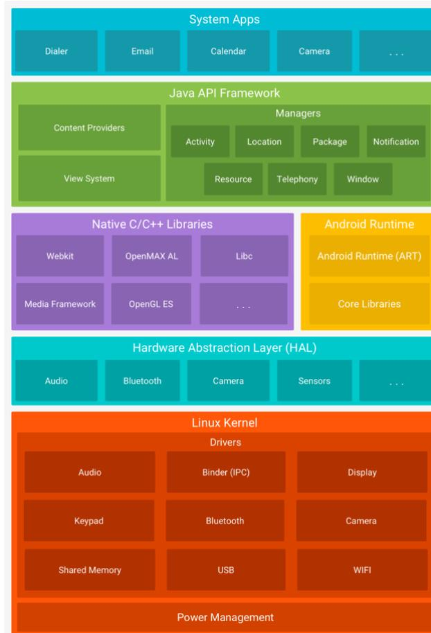
Figura 6: Pila de software de Android [11]
