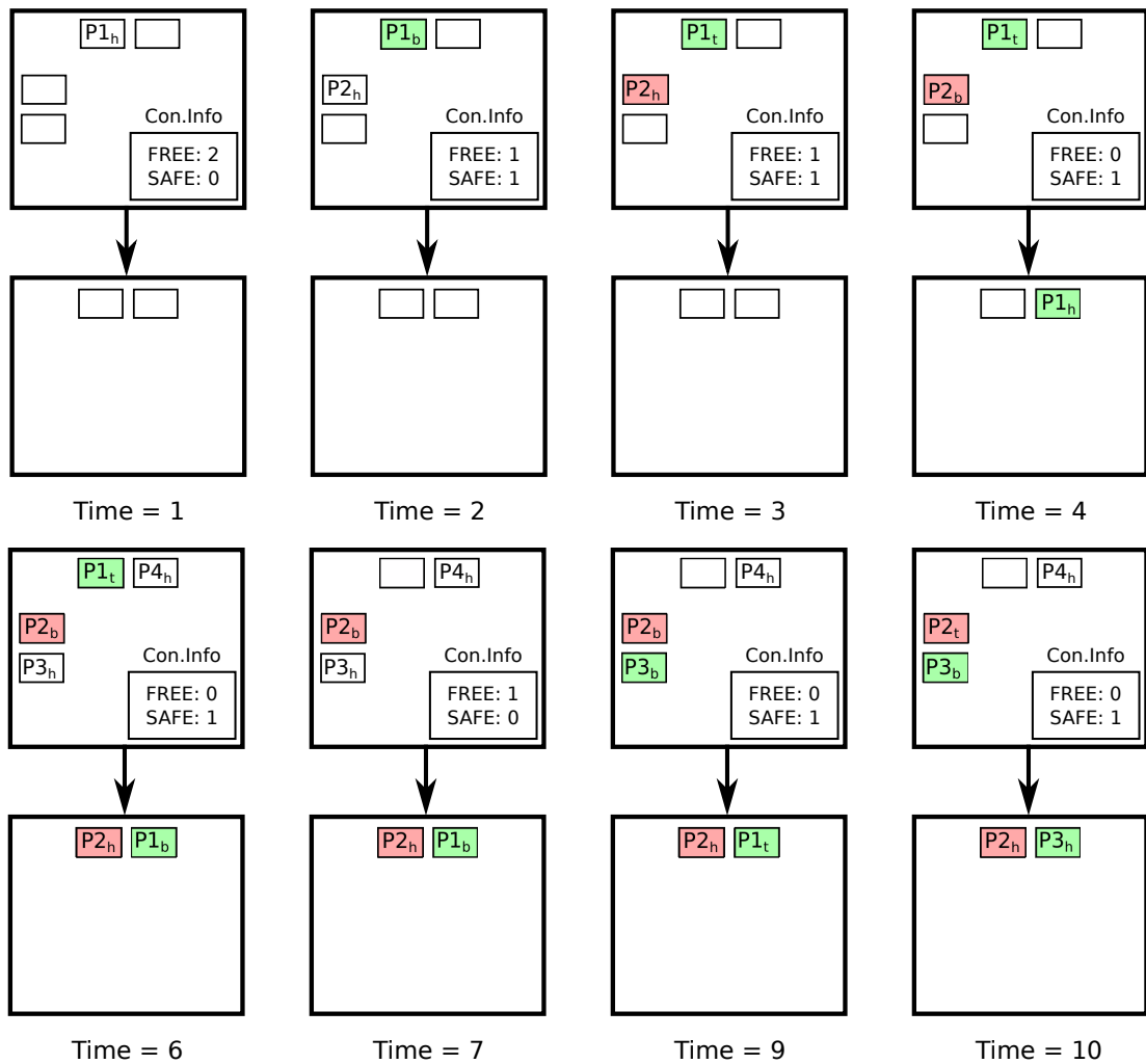
FIGURE 3.5: Logic example at the router's input port.
