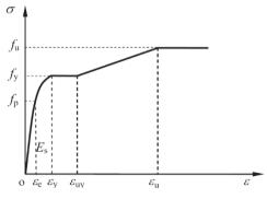
*Fig. 1.* Schematic diagram of the uniaxial stress– strain relation for steel [1].
