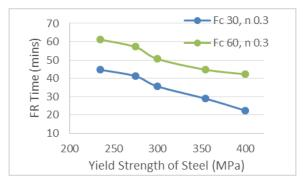
Fig. 11. FR time values for different yield strengths of steel.
