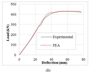
*Fig. 4.* Load–deflection curves comparison of samples (a) FAC [14] and (b) HSS-19 [15] with the FE model.
