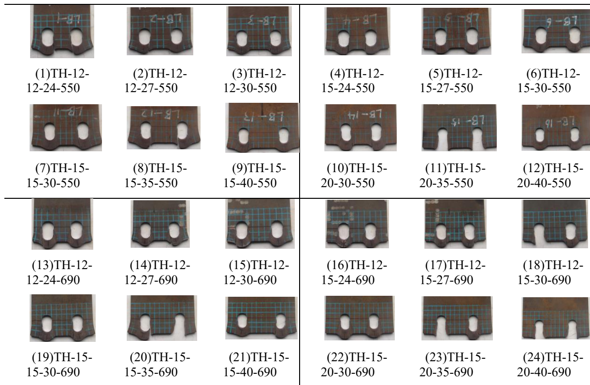
Fig. 4 Failure mode of TH connection
