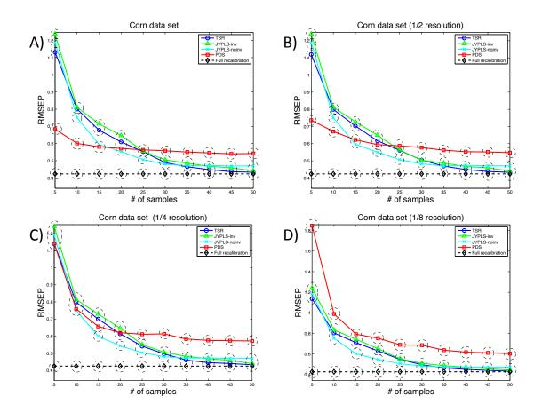
Figure 6: Corn dataset - RMSEP values obtained for the different sizes of the secondary spectrometer calibration subset with A) the same spectral resolution for both instruments, B)  $\frac{1}{2}$ , C)  $\frac{1}{4}$  and D)  $\frac{1}{8}$  of the primary instrument spectral resolution for the secondary spectrometer. Dashed ellipses mark the statistically significant differences among groups of methods (*p*-value < 0.05)
