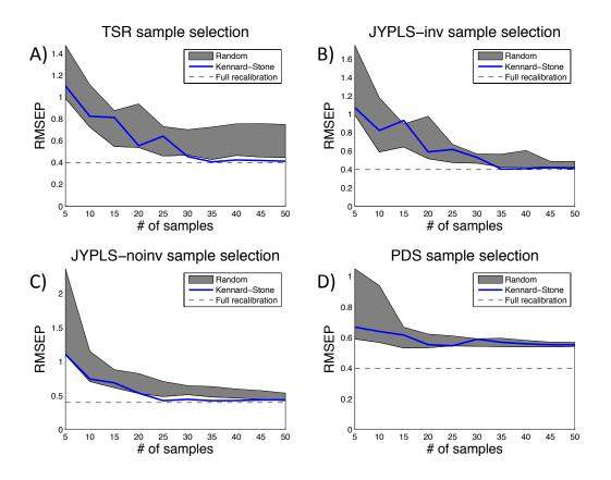
Figure 7: Corn dataset - Effect of the Kennard-Stone algorithm-based sample selection on the performance of the calibration transfer methods under study
