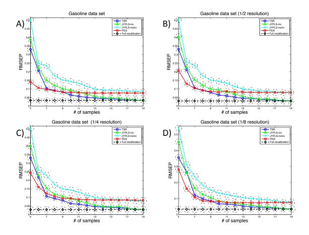
Figure 3: Gasoline dataset - RMSEP values obtained for the different sizes of the secondary spectrometer calibration subset with A) the same spectral resolution for both instruments, B)  $\frac{1}{2}$ , C)  $\frac{1}{4}$  and D)  $\frac{1}{8}$  of the primary instrument spectral resolution for the secondary spectrometer. Dashed ellipses mark the statistically significant differences among groups of methods (*p*-value < 0.05)
