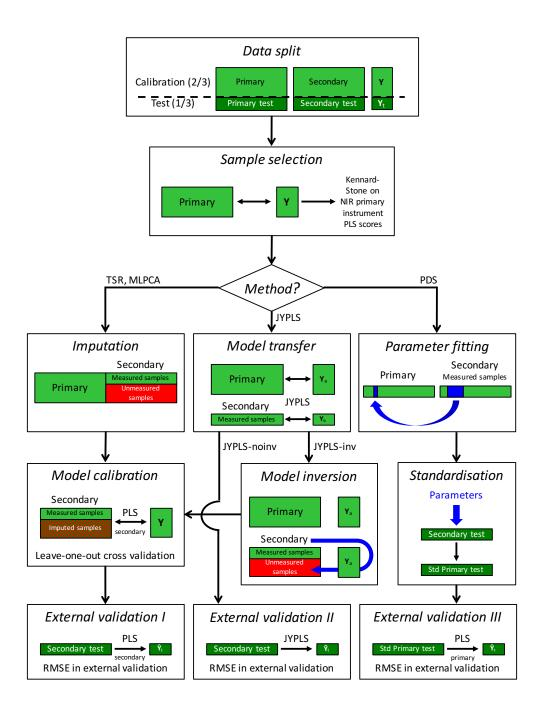
Figure 1: Flow-chart of the comparative study. Std stands for *standardised*. ^ refers to predicted values. Notice that part of the whole secondary instrument calibration set is assumed to be unmeasured when addressing the calibration transfer
