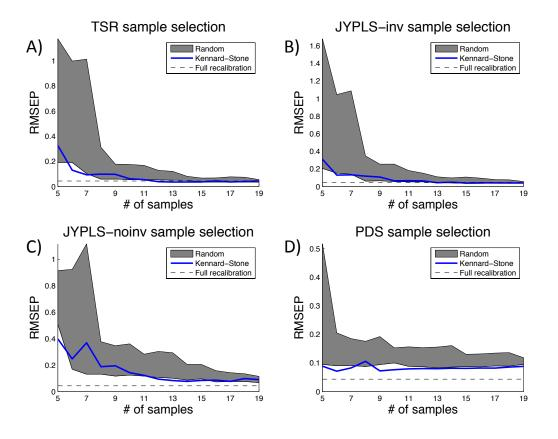
Figure 4: Gasoline dataset - Effect of the Kennard-Stone algorithm-based sample selection on the performance of the calibration transfer methods under study
