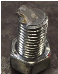
Fig. 14. Failure surface of a bolt (P3.2-1)
