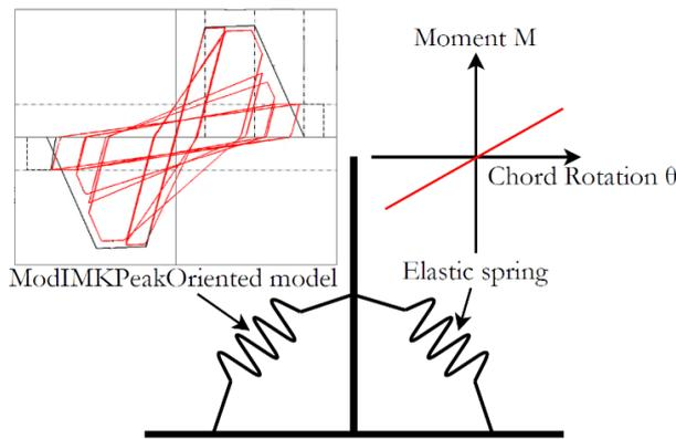
Fig. 8. The modified CP model proposed for a CFST member
