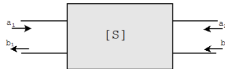
FIGURE 2.7: TWO-PORT ELEMENT OR NETWORK
