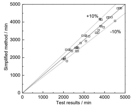
Fig. 12. Comparisons between predicted and test residual capacities
