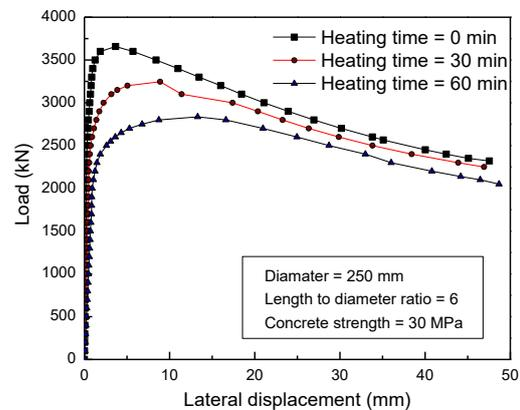
Fig. 6. Load-displacement curves [17]
