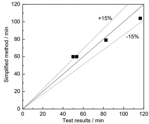
Fig. 11. Comparisons between predicted and test fire resistance
