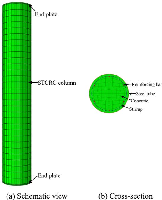
Fig. 8. FE model of STCRC columns [17]
