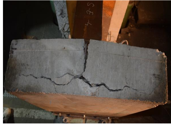
Fig. 7. Transverse bending failure (P22-T).
