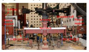
Fig. 1. Front view of quasi-static test set-up.
