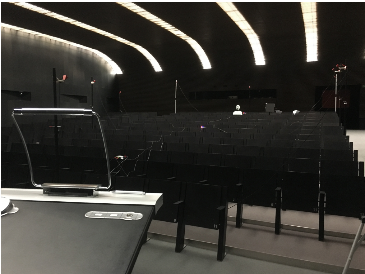
Figure 4.1: Measurement set up for a large auditorium. Infrared cameras were used to track the loudspeaker position
