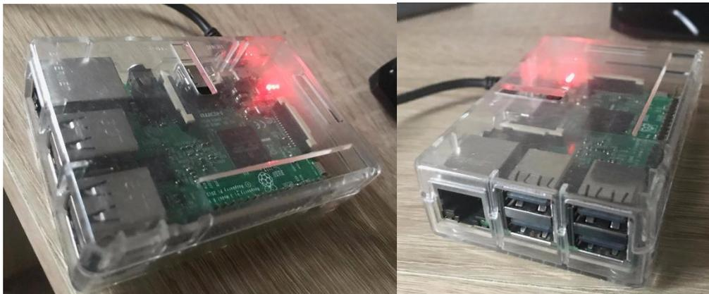
Fig. 10. RaspBerry Pi Model 3B
