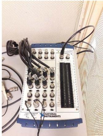
**Figura 13: Tarjeta digital NI USB-6229 BNC.**
