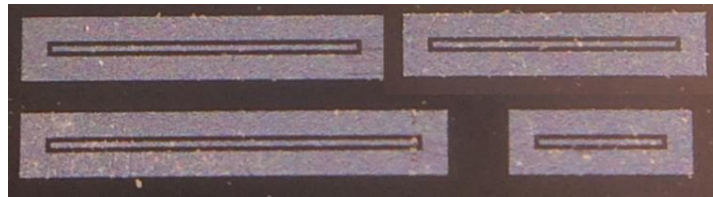
Figure 49. Fabricated CPWs with lengths between 1 mm and 3 mm.
