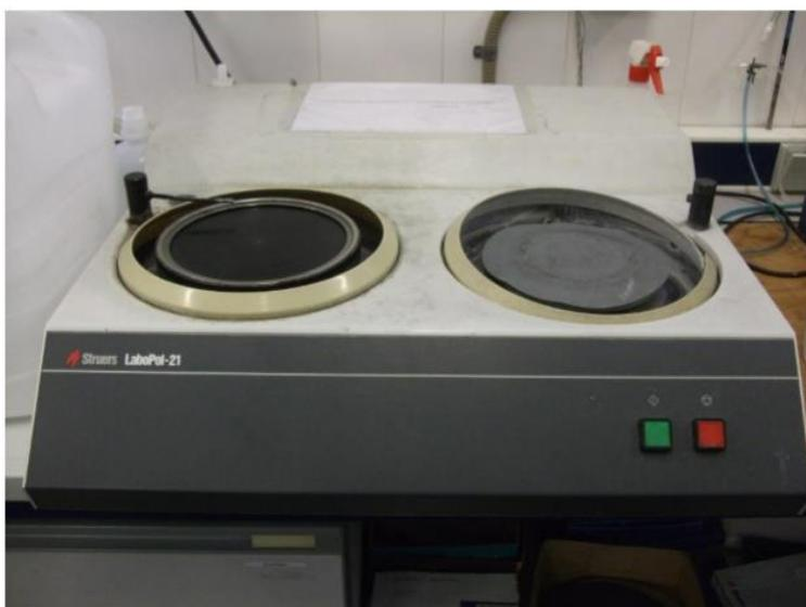
*Figura 4. Pulidora, Struers LaboPol-21*
