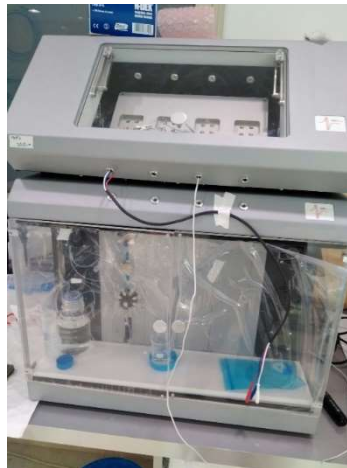
figure 20: AWS A20-F20 Research platform. Composed for an AWS A20 platform (top) where is possible see the 4 channels where the flow cells will be connected and an AWS F20 platform (down) where is possible to see the syringe, the distribution valve, the sample pump and the injection valve (bottom-top order).
