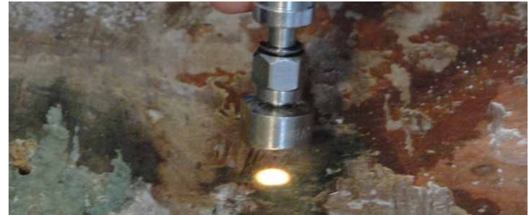
Figure 6:104. Santa Maria de Cuevas ceiling's panel FORS measurements made by Marcello Picollo and Giovanni Bartolzzi. (Photo: K. Muñoz Alcocer, 2015).
