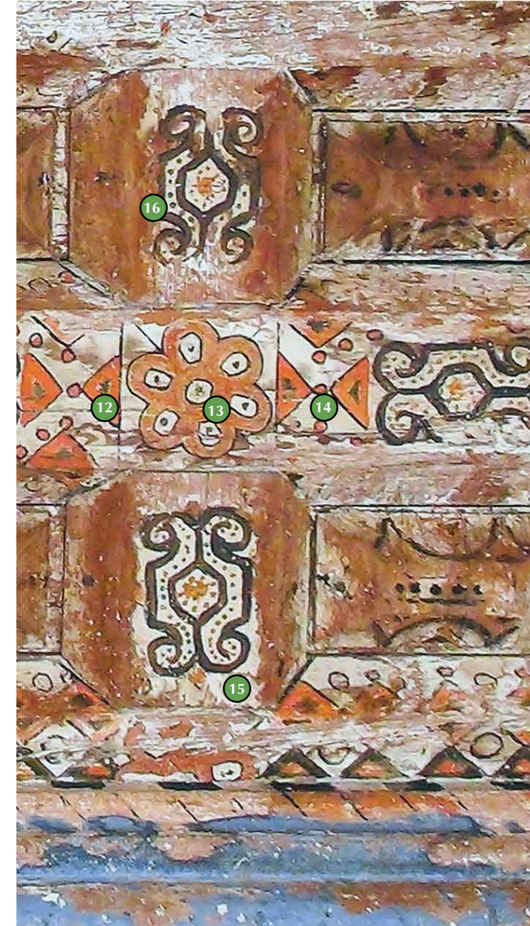
Figure 11:29. San Francisco de Borja baptistery ceiling. View of the studied area showing the analysed points by XRF and FORS. (Photo: I. Rangel, 2016. Design: L. Capitani, 2017).
