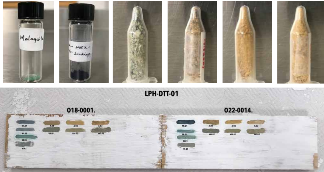
Figure 11:74. Characterization of the green colours from Santa María de Cuevas and Cusiuhiriachi ceilings. View of the materials used and the mock-ups prepared with their identification number. (Performed by: D. Maldonado, 2018).
