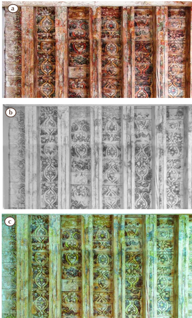
Figure 6:181. IRFC reflectography. General view of the narthex ceiling: Visible light (a); Infrared light (b); IR- False Colour image (c). (Photographs: I. Rangel Chávez, 2016).
