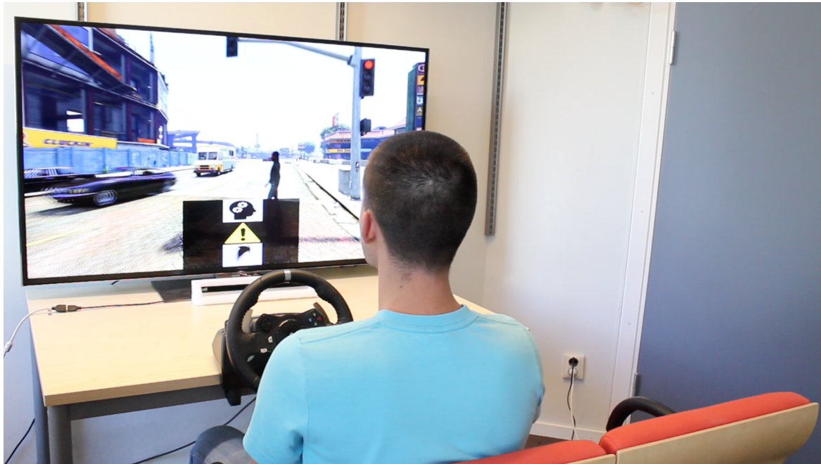
Fig. 3.3 This image shows a pedestrian shocking event, the car detects that a pedestrian is crossing in red and automatically reacts triggering the brakes.
