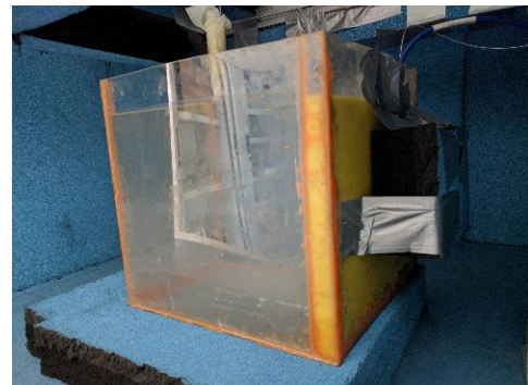
Fig. 2. Novel phantom container for phantom measurements and the on-body antenna covered with absorber
