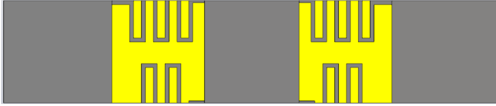
Figure 4.4. Glide symmetry of 3-layers new structure and period equal to half unit cell (Top, side and bottom view).
