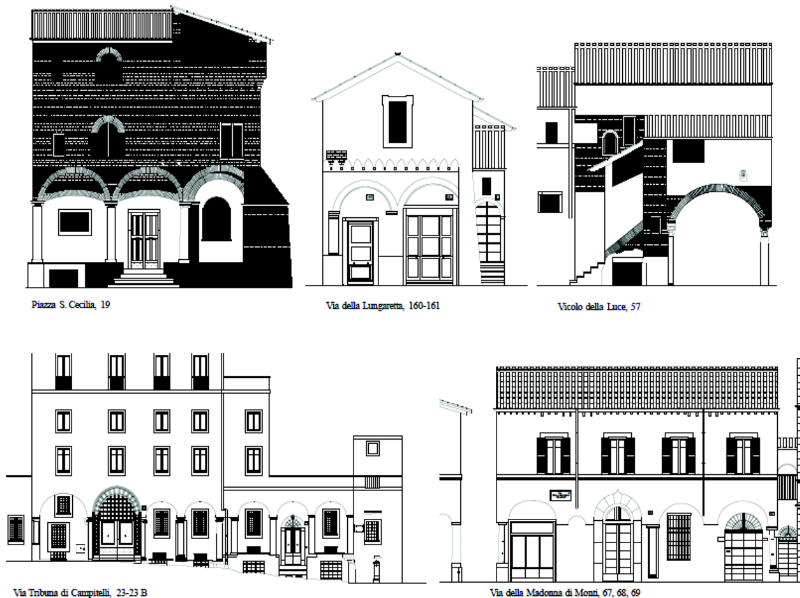
Figure 3. Type 2 arcuated façade porticoes of medieval residences in Rome
