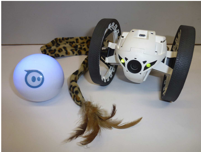
Figure 5.2: Sphero (left) and Jumping Sumo (right), the two robots used in the study.
