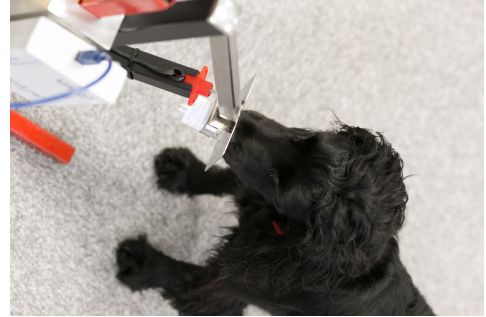
Figure 3.6: Dog using the cancer detection interface (Image courtesy of Dr. Clara Mancini)
