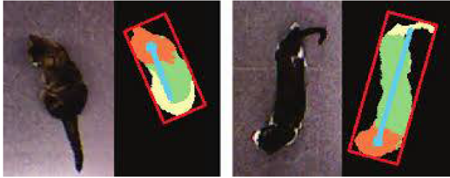
Figure 2.11: Tracking cats using depth measurement via an Xbox Kinect to detect posture [257].
