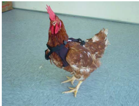
Figure 3.4: Chicken wearing a jacket which simulates human touching sensation (Image courtesy of Dr. Adrian David Cheok)
