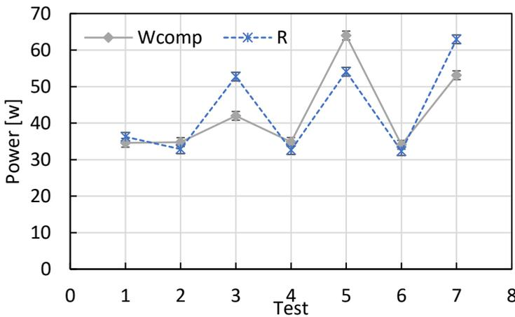
Figure 66: Compressor power and resistance power through tests campaign
