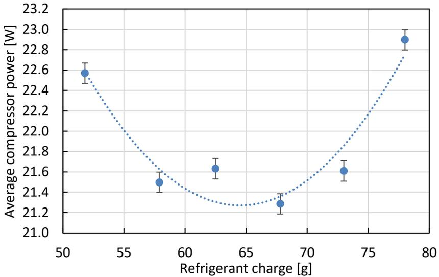
Figure 29: Average compressor power through the refrigerant charge study
