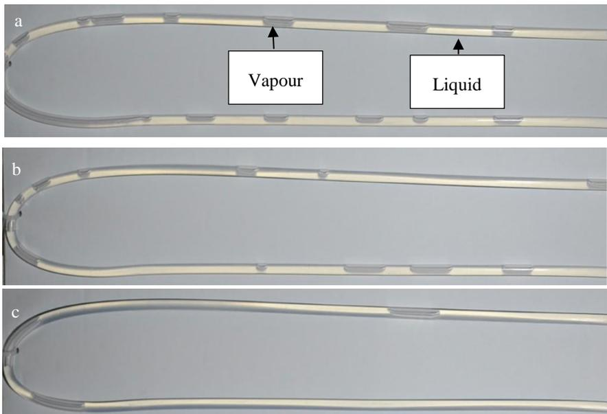
Figure 62: Condenser outlet for different compressor speeds a) 1800 rpm b) 2500 rpm and c) 3500 rpm
