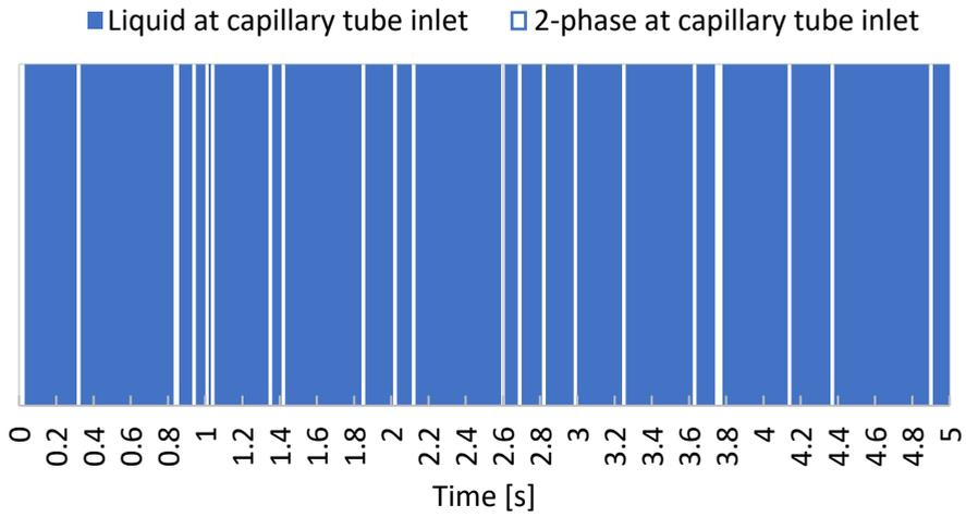
Figure 61: Liquid level evolution at the capillary tube inlet for tests 2 and 6
