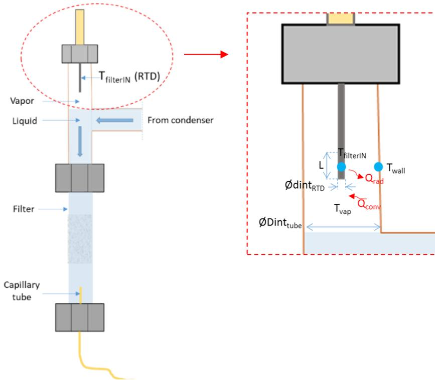
Figure 57: Heat exchange inside refrigerant circuit
