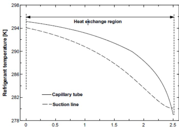
Figure 15: Example of reverse heat transfer [18]
