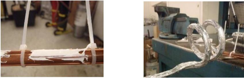
*Figure 22: Set up of the three capillary tubes around the suction line*
