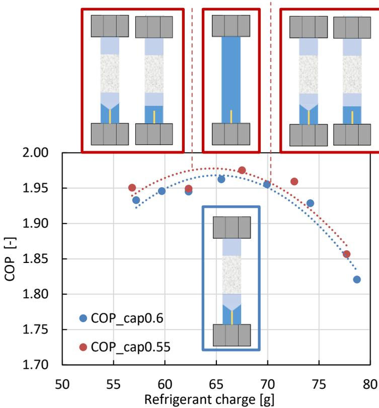
Figure 72: COP and liquid level inside filter for different refrigerant charges for the two tested capillary tubes, of 0.55 mm and 0.6 mm diameter respectively
