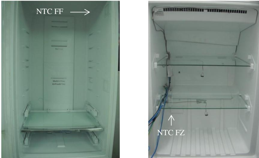
Figure 7: NTC location inside FF and FZ cabinets
