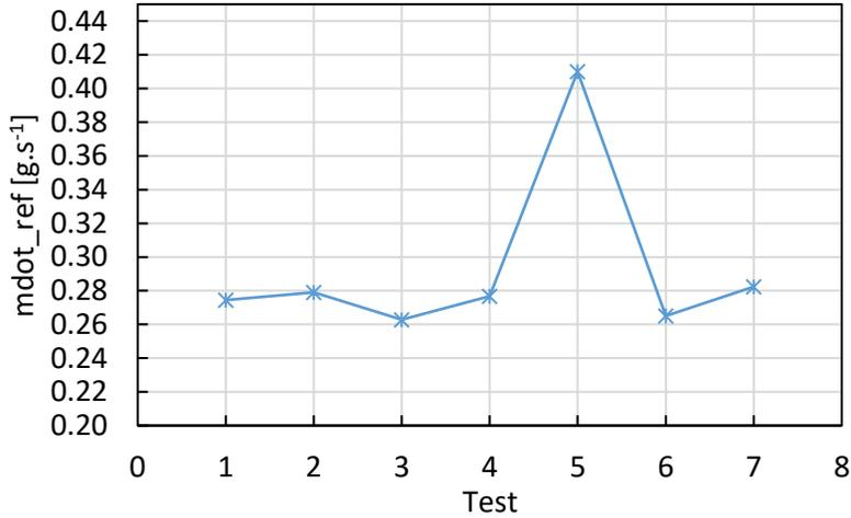
Figure 64: Refrigerant mass flow rate through tests campaign
