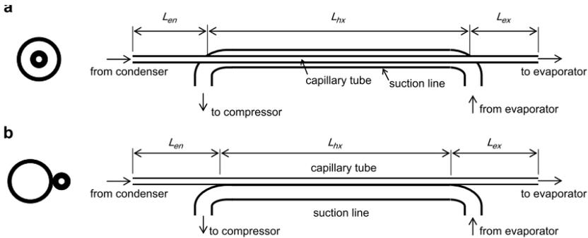
Figure 10: Schematic of the capillary tube-suction line heat exchanger: (a) concentric, (b) lateral [21]
