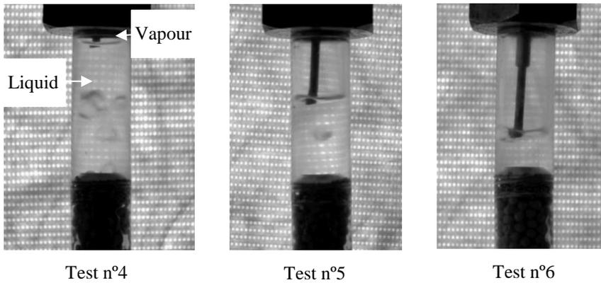
Figure 36: Capillary tube inlet for tests 4, 5 and 6
