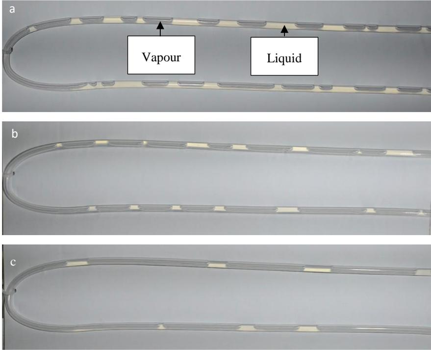
Figure 46: Visualisation of the condenser outlet with a)  $\dot{m}_w=0.447 \text{ kg}\cdot\text{min}^{-1}$
