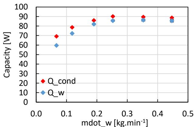
Figure 47: Water and condensing capacities varying water mass flow rate
