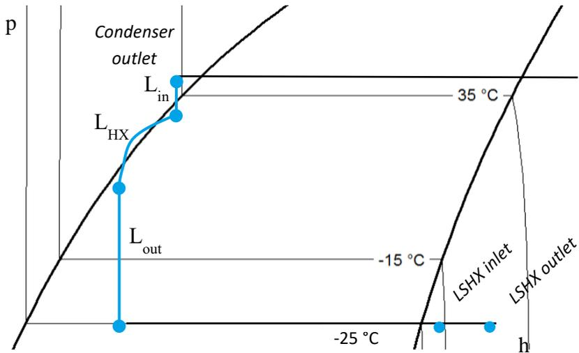
Figure 13: Pressure-enthalpy diagram of recondensation phenomenon in CT-LSHX
