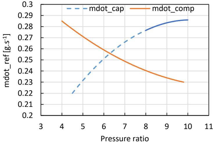
Figure 54: Refrigerant mass flow rates matching
