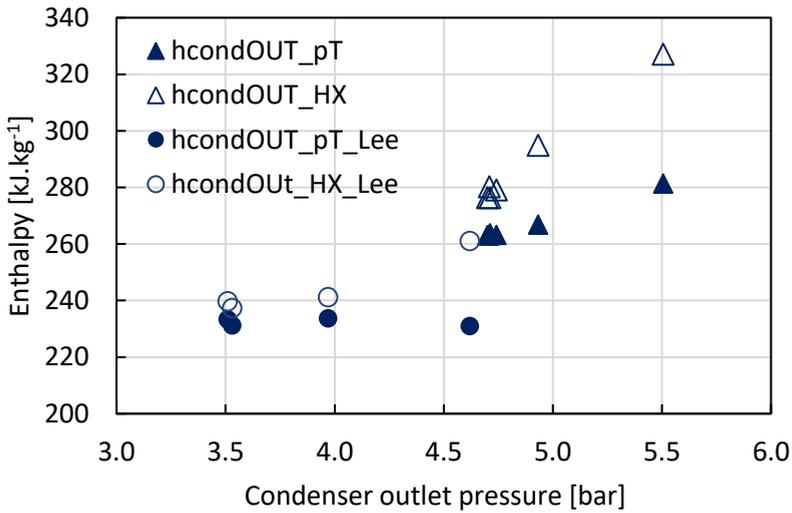
Figure 53: Enthalpies evaluated from the pressure and temperature measurements and the assumption of thermodynamic equilibrium, and enthalpy evaluated from the inlet refrigerant conditions and the heat measured on the water side compared with data obtained by Lee et al. [16].
