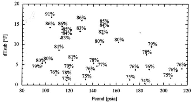
Figure 21: Effectiveness for different operating conditions with respect to subcooling [13]
