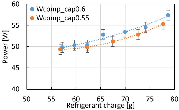
Figure 73: Compressor power for different refrigerant charges for the two tested capillary tubes, of 0.55 mm and 0.6 mm diameter respectively
