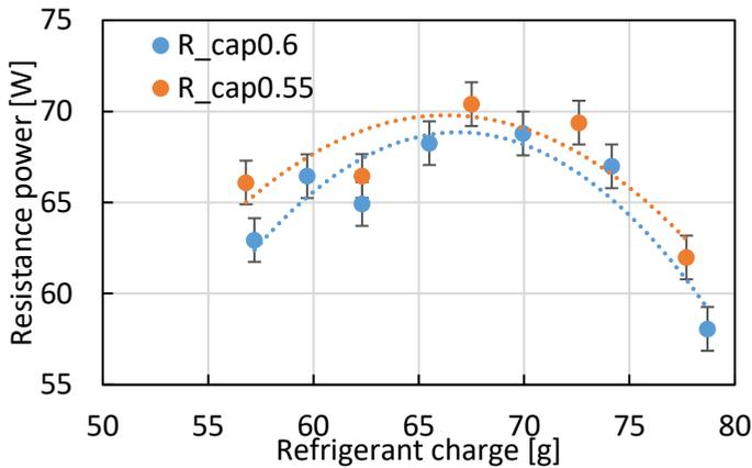
Figure 75: Resistance power of 0.55 mm diameter and 0.6 mm diameter capillary tubes for different refrigerant charges
