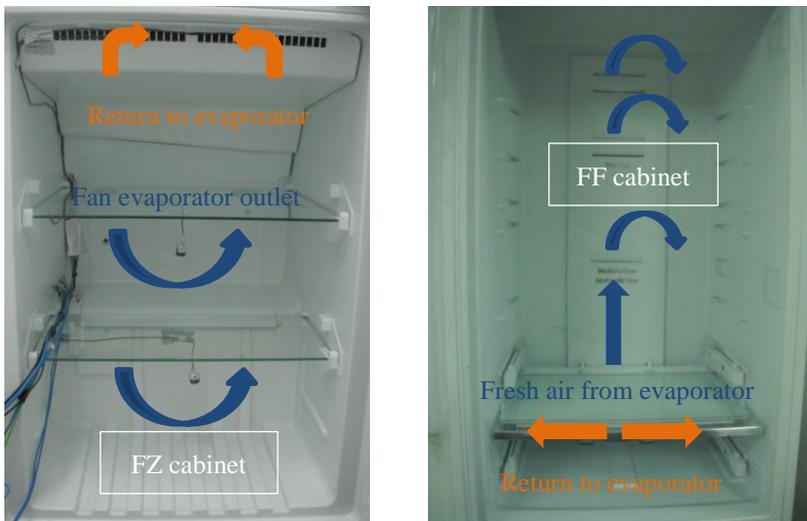
*Figure 6: Air distribution in FF and FZ cabinets*
