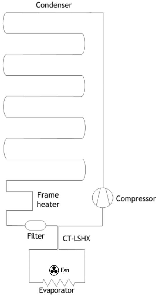
*Figure 1: Refrigerant loop of a household refrigerator*
