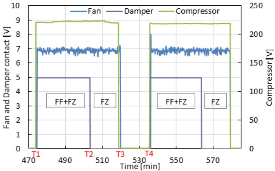
Figure 28: Identification of time parameters for the calculation of the compressor energy consumption during a typical refrigeration dynamic cycle
