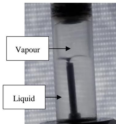
*Figure 45: Two-phase flow capillary tube inlet*
