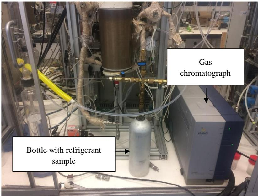
*Figure 44: Gas chromatograph experimental set up*
