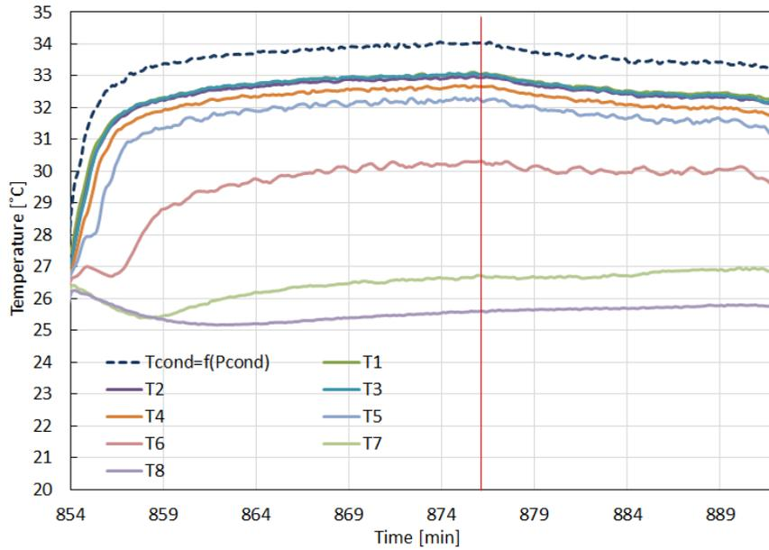
Figure 31: Temperatures along the condenser for 73 g refrigerant charge
