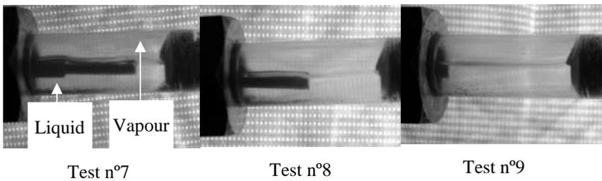
Figure 37: Capillary tube inlet for tests 7, 8 and 9
