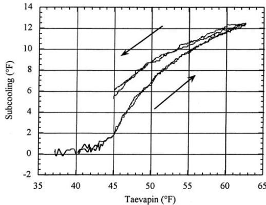
Figure 17: Hysteresis effect of mass flow rate versus subcooling [13]
