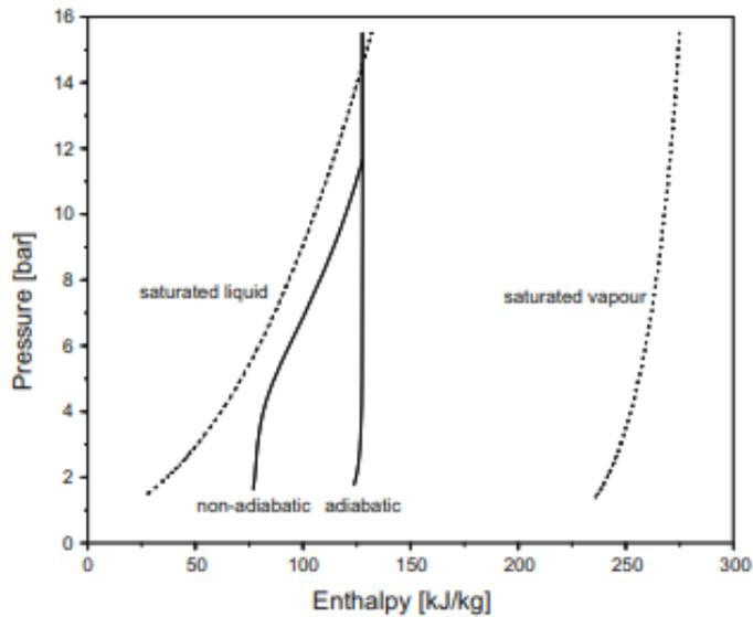
Figure 9: Flow pattern of non-adiabatic vs. adiabatic capillary tube [21]
