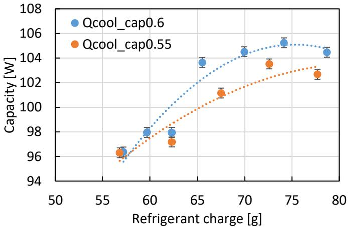
Figure 74: Refrigerant cooling capacity for different refrigerant charges for the two tested capillary tubes, of 0.55 mm and 0.6 mm diameter respectively
