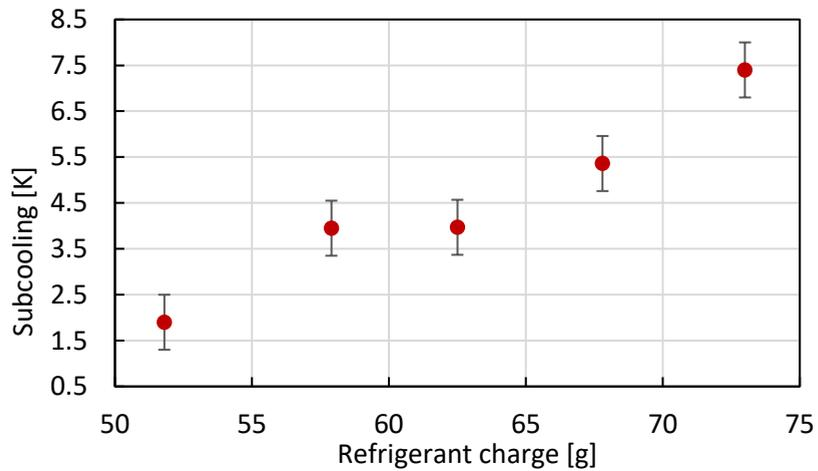
Figure 32: Evolution of subcooling through the refrigerant charge study
