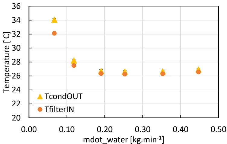
Figure 51: Comparison between condenser outlet temperature and capillary tube inlet temperature
