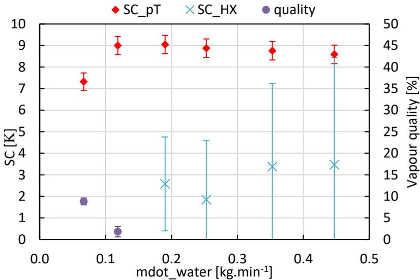
Figure 50: Subcooling evaluated from the pressure and temperature measurements and the assumption of thermodynamic equilibrium, and subcooling evaluated from the inlet refrigerant conditions and the heat measured on the water side.
