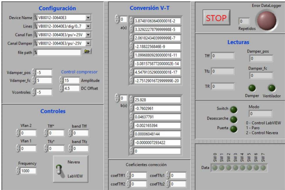
Figure 39 : Labview platform interface
