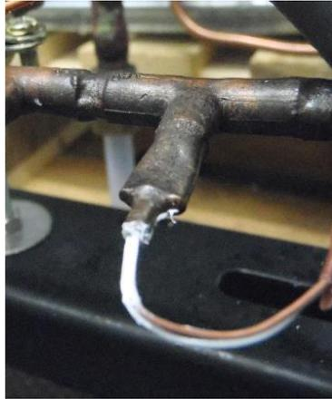
Figure 25: Outlet condenser temperature measurement
