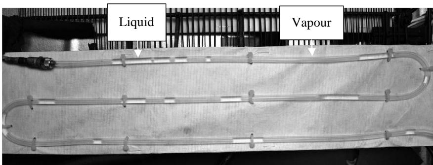
*Figure 33: Refrigerant flow at the condenser outlet*
