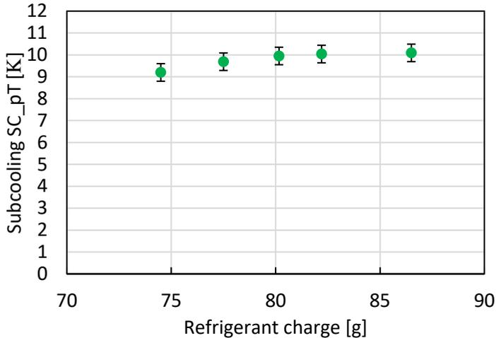
Figure 42: Subcooling for different refrigerant charges
