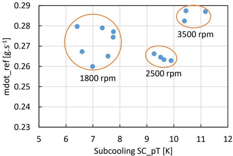
Figure 68: Mass flow rate variation vs.  $SC_{PT}$  measured subcooling for different compressor speeds
