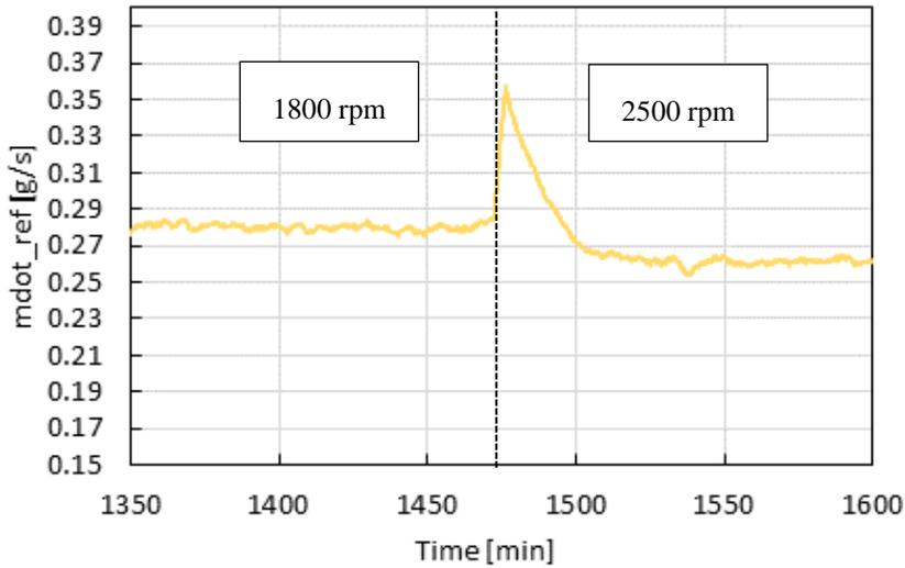
Figure 69: Change in refrigerant mass flow rate from 1800 rpm to 2500 rpm
