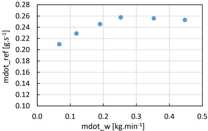
Figure 49: Refrigerant mass flow rate vs. water mass flow rate
