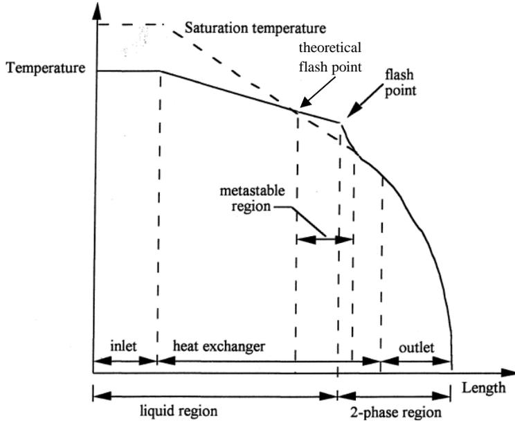
Figure 12: Refrigerant flow through capillary tube, adapted from [13]
