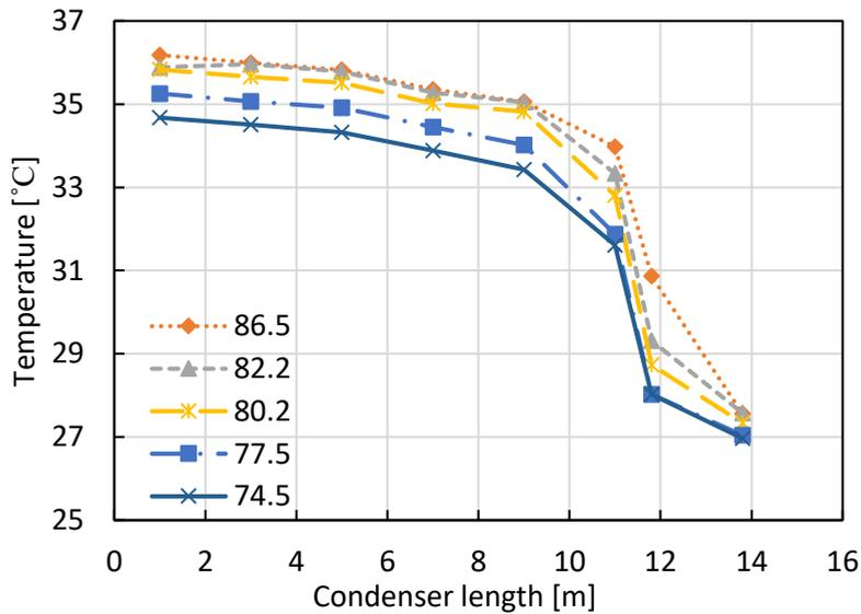
Figure 43: Temperature along condenser for different charges tested
