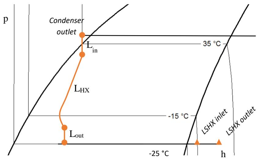
Figure 16 : Pressure-enthalpy diagram of reverse heat transfer phenomenon in CT-LSHX
