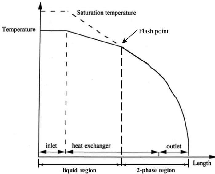
Figure 11: Evolution of refrigerant temperature along the capillary tube, adapted from [13]
