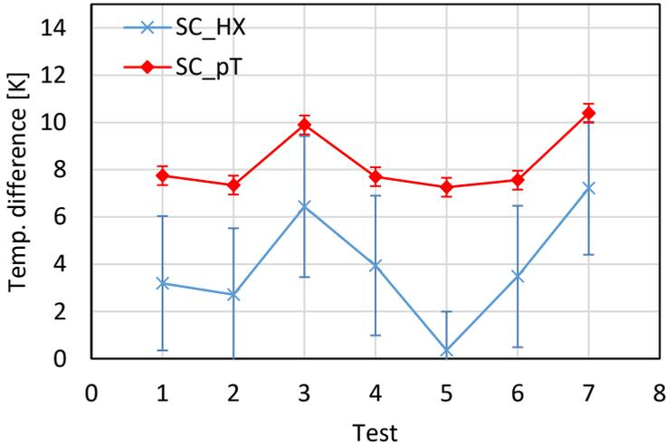
Figure 63: Subcooling evaluated from the pressure and temperature measurements and the assumption of thermodynamic equilibrium ( $SC_{pT}$ ), and subcooling evaluated from the inlet refrigerant conditions and the heat measured on the water side ( $SC_{HX}$ )
