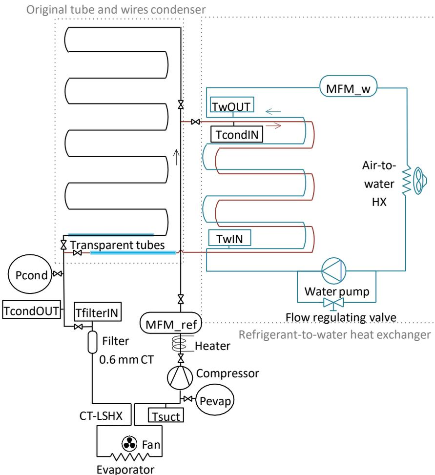
Figure 38: Diagram of the tests bench
