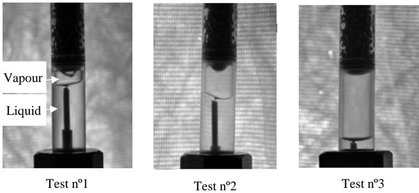
Figure 35: Capillary tube inlet for tests 1, 2 and 3
