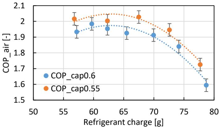
Figure 76: COP using air cooling capacity of 0.55 mm diameter and 0.6 mm diameter capillary tubes for different refrigerant charges
