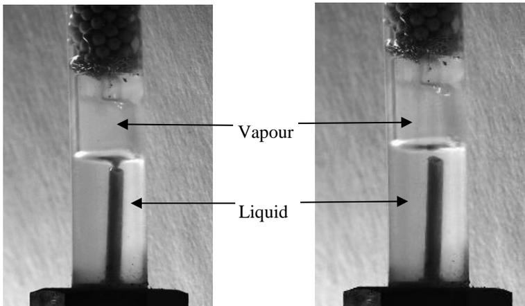
b) Two-phase flow liquid inlet at 1800 rpm: tests 2 and 6
