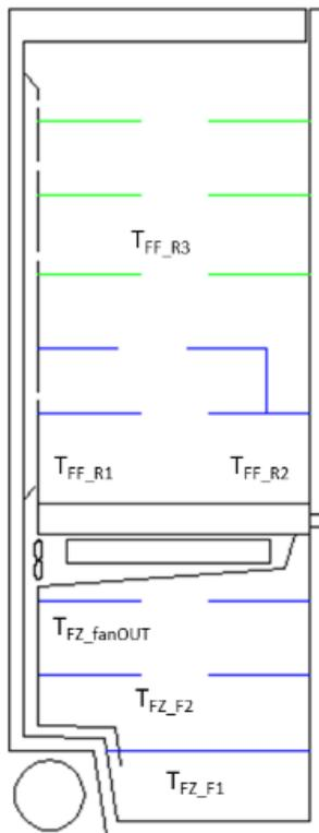
Figure 26: Air FF and FZ temperatures measurement locatio
