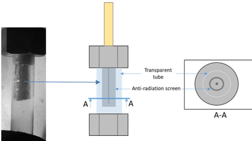
Figure 58: Set up of the anti-radiation shield around the RTD
