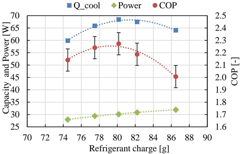
Figure 41: Cooling capacity, COP and compressor power for different refrigerant charges
