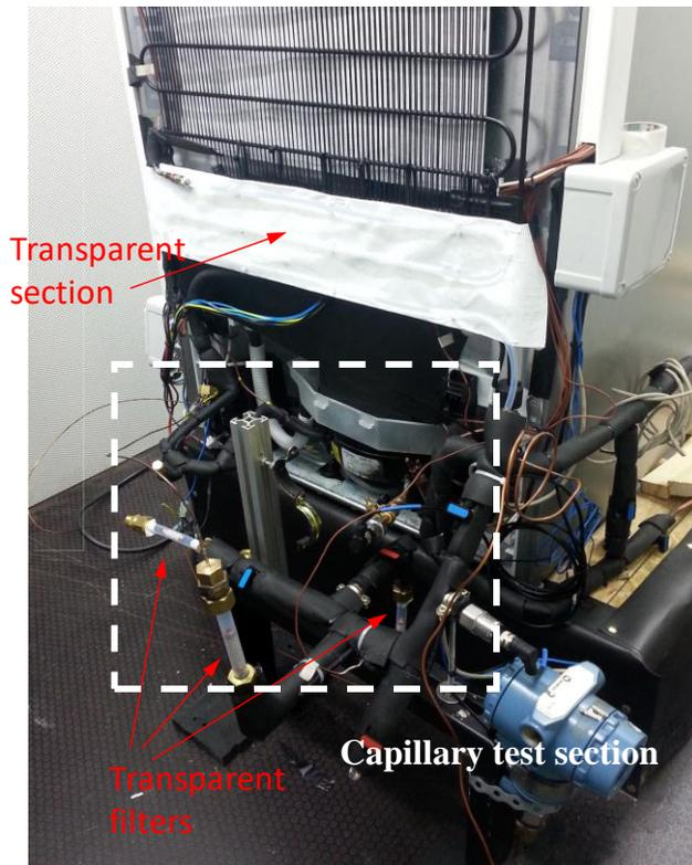
*Figure 23: Visualisation test bench*
