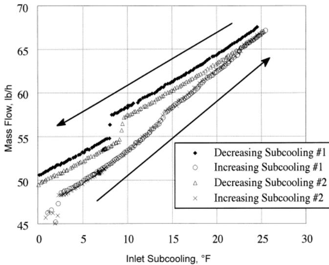
Figure 67: Hysteresis in the capillary tube mass flow rate [26]
