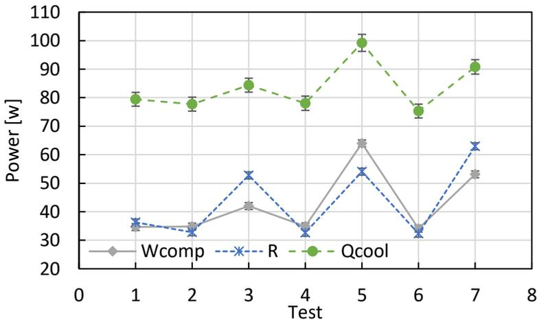
Figure 70: Evolution of cooling capacity, resistance power and compressor power across the tests
