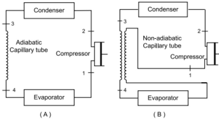
Figure 8: Set up of adiabatic (A) vs. non-adiabatic (B) capillary tube [20]
