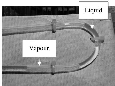
*Figure 34: Refrigerant flow in a condenser bend*
