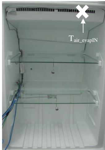
*Figure 56: Air evaporator inlet thermocouple location*
