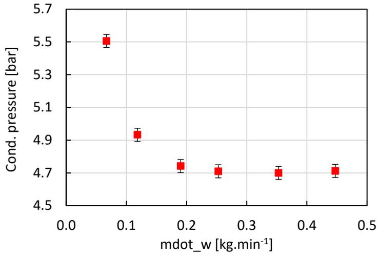
Figure 48: Condensation pressure vs. water mass flow rate
