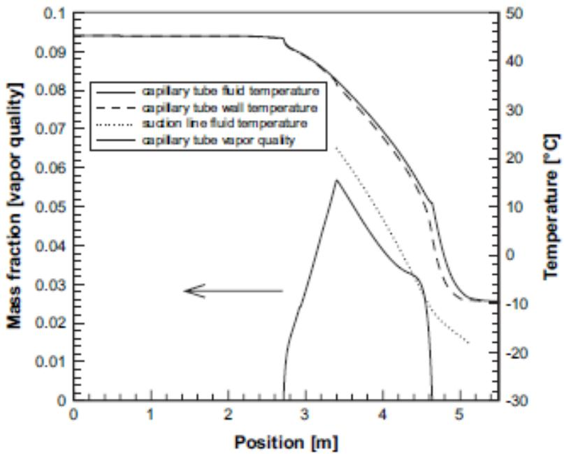
Figure 14: Example of recondensation phenomenon [33]
