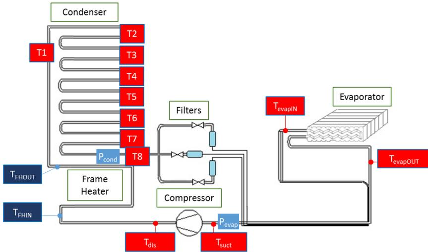
Figure 24: Refrigerant temperature and pressure measurements location
