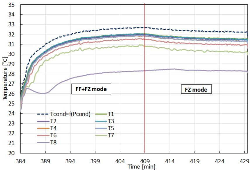
Figure 30: Temperatures along the condenser for optimal refrigerant charge (62.5 g)
