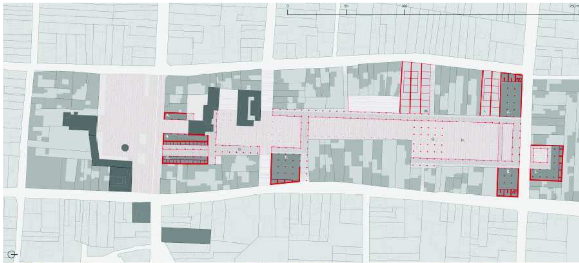
A municipality offices; B. library; C. Market; D. New public space in connection with the school patio; E. arcade, public urban space with flexible use, result of the overlapping of the urban routes into the block; F. public equipment, multi-use building; G. hypostyle space with retractable roof; H. square, open air public space; I. Proposal of substitution and updating of the housing building; J// K. public equipment, multi-use building; L. public equipment, handicraft exhibition building; M. commercial spaces;
