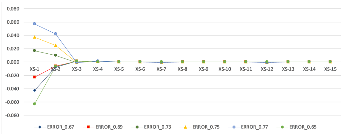
Figure 16. Sensitivity analysis based on the potential error in the water surface elevation (WSE) at the first transect.
