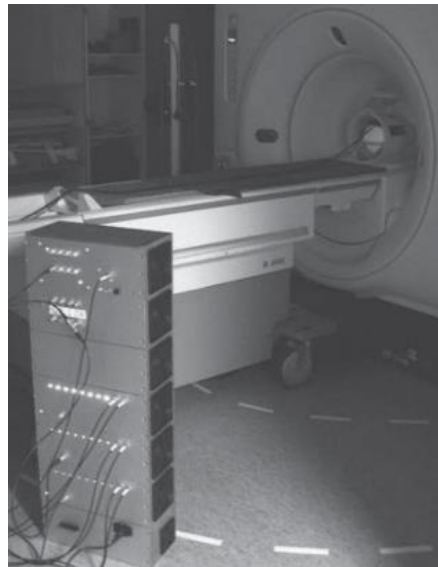
Figure 7: MR-compatible NIRS device in a 1.5-T MRI room [14].
