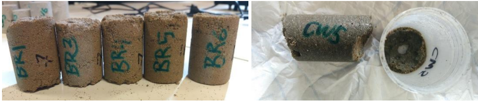
Figure 32: Pictures of specimens of mortars with 100% of dehydrated CEM I from SECIL and sodium carbonate 1M (left) and 25% of slag, 75% of dehydrated CEM I from SECIL and water (right)
