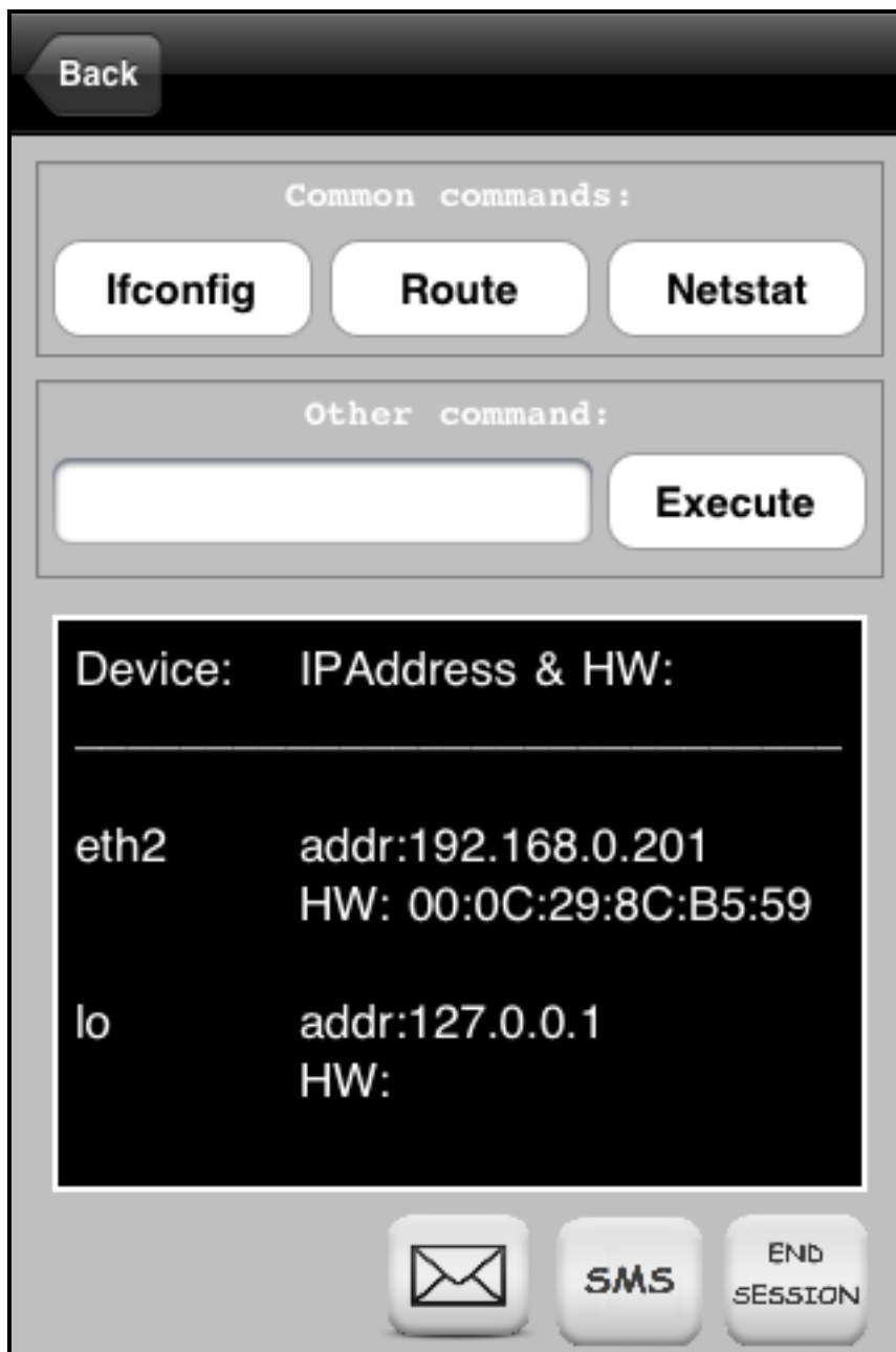
Picture 4 – 13. Ifconfig parsed command.
