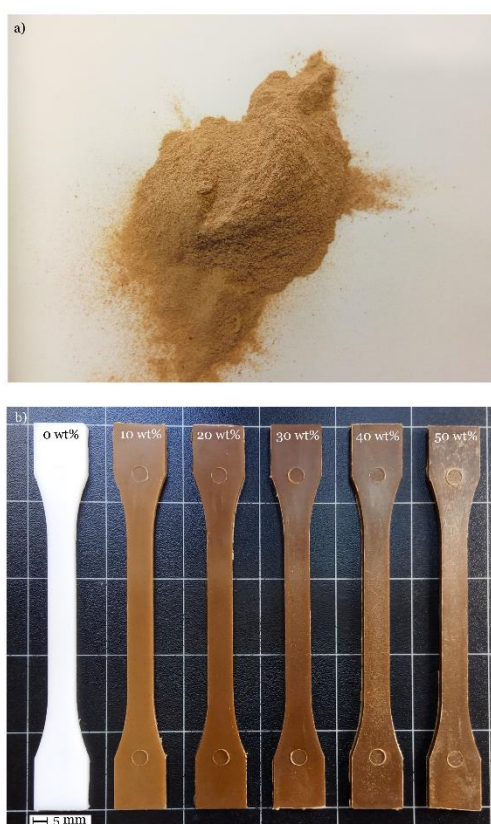
Figure III.3.1. a) Powdered almond shell flour (ASF) and b) injection moulded PBS/ASF/MLO composites with varying ASF content in wt%.
