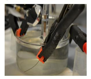
Fig. 1. Experimental setup for impressed current cathodic protection: a) General view of the cathodic protection system; b) Cathodic protection of the right and left string. Central string without protection; c) End of the protected string immersed in 0.1 M KNO<sub>3</sub>.
