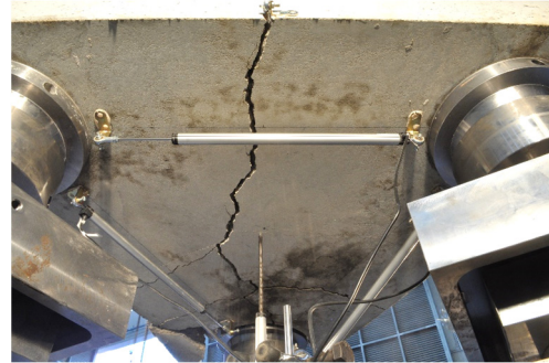
CARA INF – Colapso
