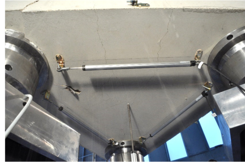
CARA INF – Colapso
