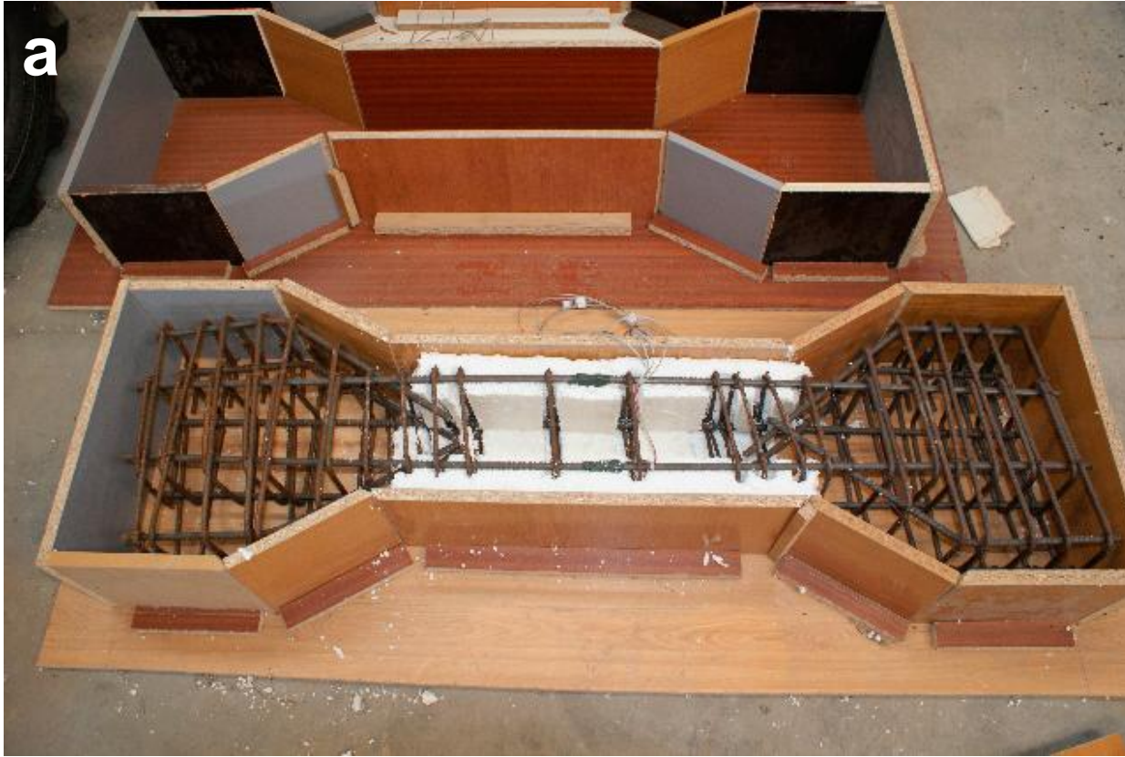
Fig. 2. a) Specimen contained by formwork; b) Damaged Column (DC) before repair.
