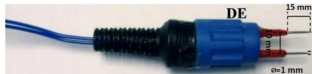
Figure 2. Stainless steel double-needle sensor [33].
