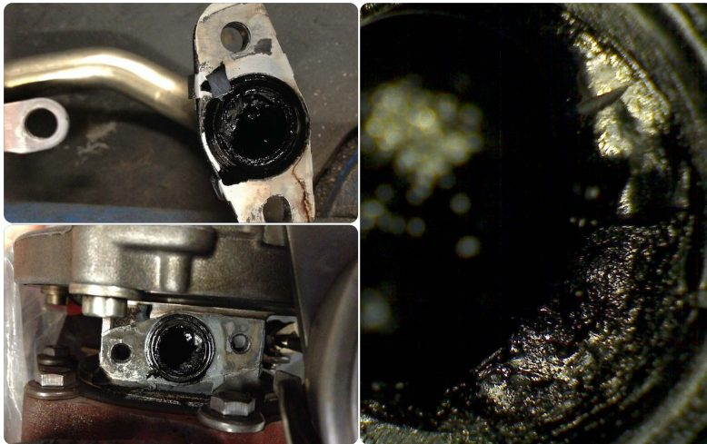
Figure 4.17: Oil coke deposits in a turbocharger tested at 2750 rpm- full load and oil “A” at 7% soot
