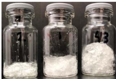
Fig 1 Vacuum-foam dried (VFD) preparations of 15%, 30%, and 40% sucrose (left to right).
