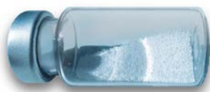
Fig. 4 Spray Freeze-Dried microspheres generated for a 20% (w/w) sucrose solution.
