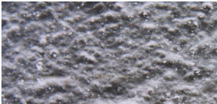
Figure 2. SEM microphotograph of the original geomembrane at \times 90 magnification
