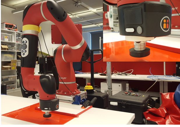
Fig. 2 Experimental setup: 7R serial manipulator with a force sensor attached to the robot end-effector, a tool consisting of a cylinder and a flat rectangular plastic object as target
