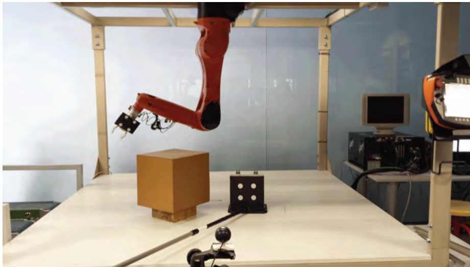
Figure 9.: Experimental setup: 6R serial industrial manipulator in ceiling position with markers in the tool and the warehouse, camera out of the robot (eye-to-hand), obstacle and robot PC.
