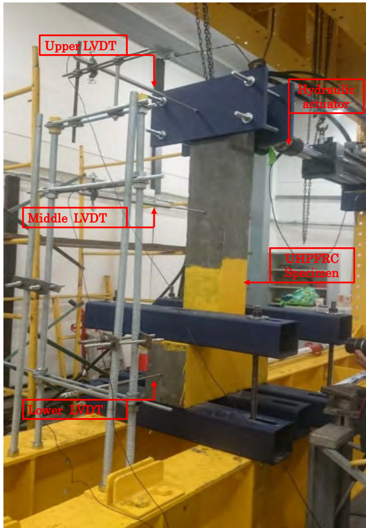
Figure 3. Set-up of the cyclic load test.
