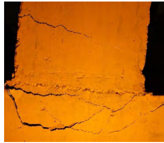
Figure 11. Evolution of the damage (cracking) in the specimens for different drift ratio.
