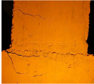
Figure 11. Evolution of the damage (cracking) in the specimens for different drift ratio.
