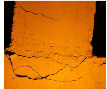
Figure 11. Evolution of the damage (cracking) in the specimens for different drift ratio.
