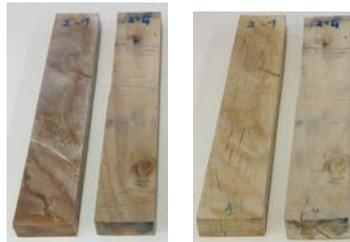
**Fig.6: Effect of continuous microwave drying of wood at 500 W; Before and after drying.**
