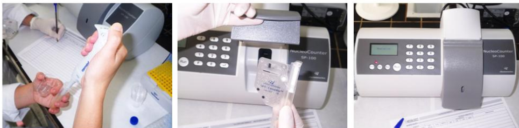
Figure I.3. Nucleocounter SP-100 (Chemometec, Allerød, Denmark) for determining sperm concentration.
