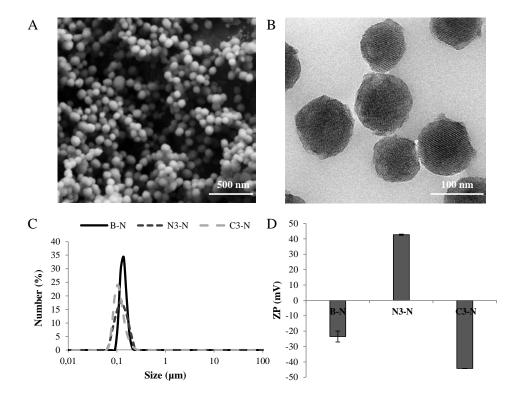
**Figure 1.** Material characterization of bare and functionalized MCM-41 nanoparticles. FESEM (A) and TEM (B) images of bare nanoparticles. The size distribution (C) and zeta potential (D) of bare and functionalized MSNs dispersed in RB.
