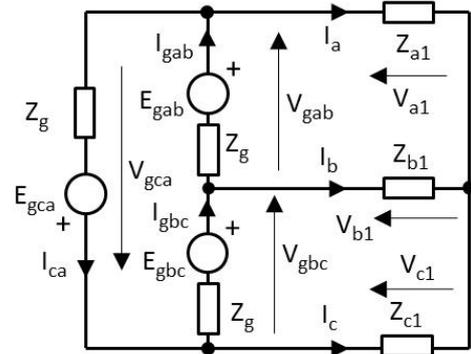
Fig. 5. Three-phase electrical system with delta-connected generator and star-connected load.
