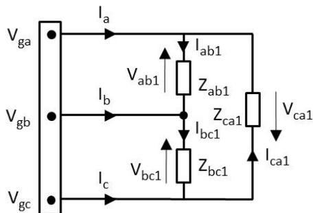
Fig. 3. Three-phase electrical system with star-connected generator and delta-connected load.
