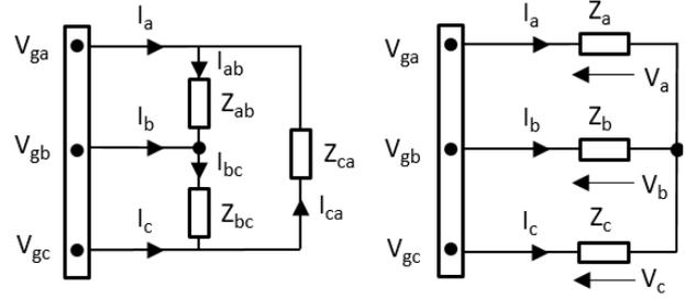
**Fig. 9.** Original circuit with delta-connected load and its star-connected equivalent.
