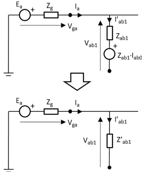
Fig. 4. Initial and equivalent circuit.
