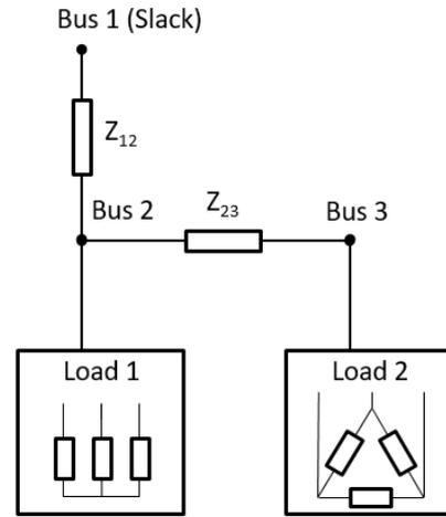
Fig. 11. Three-wire three-bus electrical system with two unbalanced three-phase linear loads.
