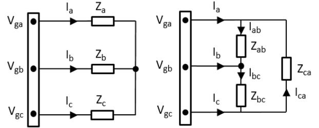
Fig. 7. Original circuit with star-connected load and its delta-connected equivalent.
