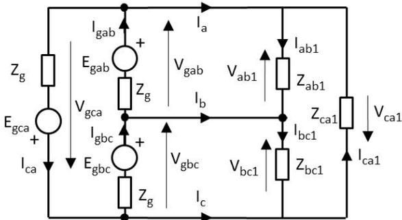
Fig. 6. Three-phase electrical system with delta-connected generator and delta-connected load.
