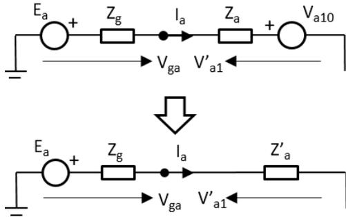
Fig. 2. Initial and equivalent circuit.
