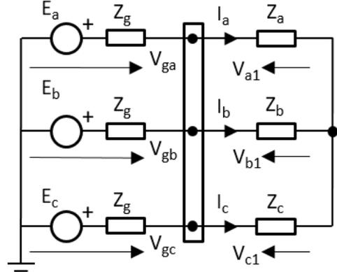
Fig. 1. Three-phase electrical system with generator and star-connected load.
